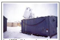
In 1999, this equipment was used to estimate haze in Barrow, Alaska. It measured how much light was being scattered by particles floating in the air.
